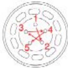
Correct tightening order for wheel bolts
