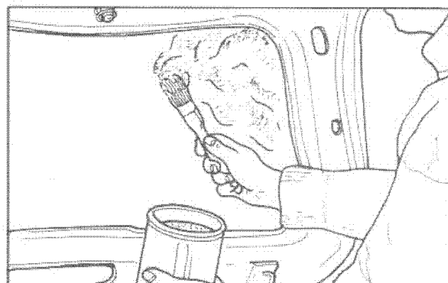
Fig. P:23 Applying adhesive to bonnet
